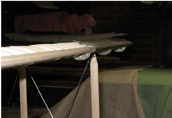
The wing slats that created some problems.
