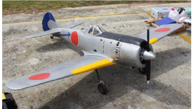
Model Engines did not have a large representation this year but Neil Addicott flew this Nakajima Ki-43 powered by a OS 70cc, seven cylinder, four stroke radial engine.
