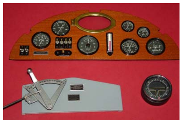
Instrument panel with the porthole between the cockpit and cabin, the throttle quadrant and the compass.
