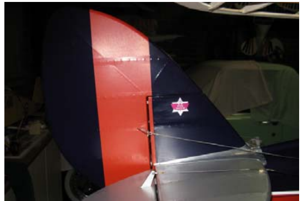
Scale rudder and elevator control wires and horns.
