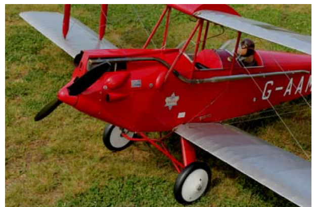
Robert Zyp from NSW, who is renowned for his magnificent model reproductions of early biplanes, had this 1/3 scale De Havilland 60G Gipsy Moth. Model spans 3.1m, weighs 16kg and is powered by a MVVS 58 two stroke petrol engine.
