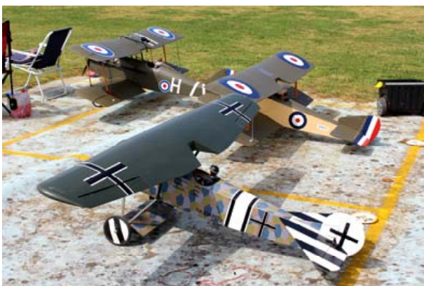
David Foster from NSW brought this collection of WWI scale models. All are from Balsa USA kits to 1/4 scale and covered with Solartex. The S.E.5 and Sopwith Pup are powered by Laser 150 four strokes and the Fokker DVIII by a CRRC 26cc petrol engine.
