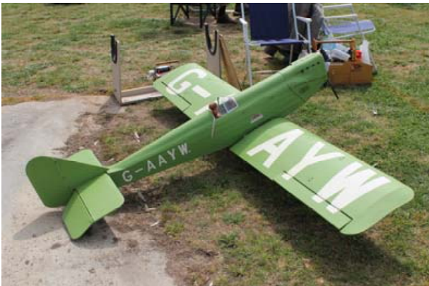
Avro Avian by Doug Radford of the Warringah club in NSW is 1/4 scale, scratch built from a smaller magazine plan. Model is 2.31m span, and is very light at 5.5kg. Powered by an early OS 120 four stroke.
