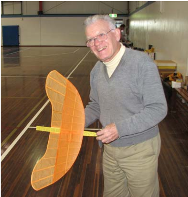
Gary Sunderland with his model based on Igo Etrich's early experiments with aircraft designs derived from the seed of the Zanonía palm .
