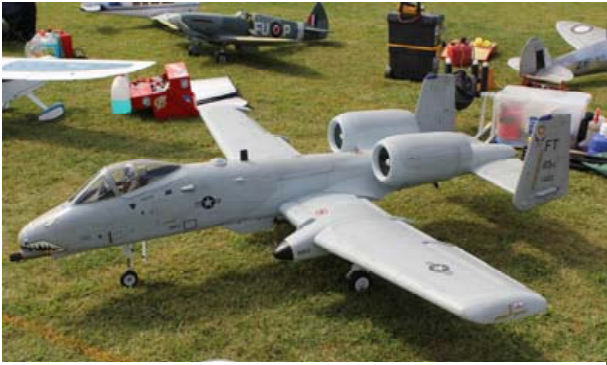
Rowdy Matthews from South Australia had three models on show. This one is a A-10 Warthog ARF by Fly Eagle Jet. Model spans 2.64m and weighs 28kg. Power is by two ATJ 120 turbines producing 26kg of thrust.
