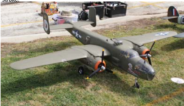
A B-25 Mitchell modified from the original ESM ARF kit by Ron Clark from NSW. Model is 2.41m span, weighs 14kg and is powered by two MVVS 26cc two stroke petrol engines.
